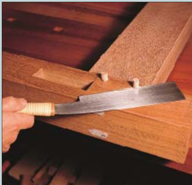
Cutting of excess with flush cut saw
