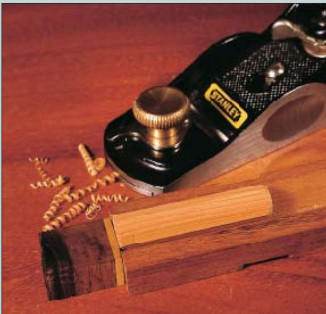
Dowel blank being planed octagonal in V-shaped cradle
