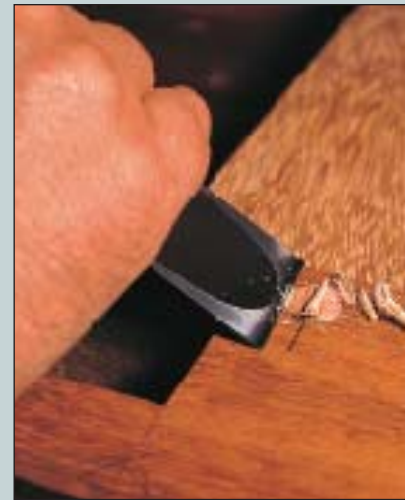
Bevelling the peg so that it will not split while being planed
