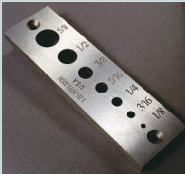
Lie-Nielsen dowel plate, A2 alloy hardened to Rockwell 60-62c
