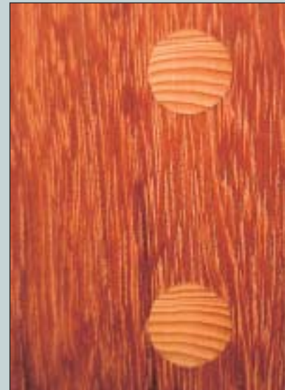
Yew pegs in Pau Rosa. Note that the growth rings are lined up neatly
